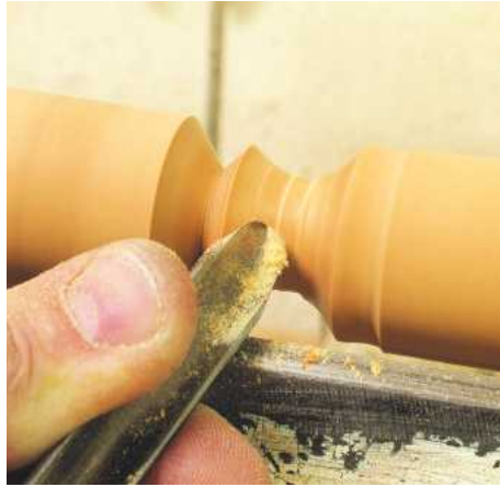
▲ Pic.20 The small gouge is used for cutting the coves. The small bevel will only put a small amount of pressure onto the timber. A long stem can be built up with a series of these shapes
